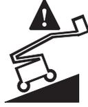
**ANSI, CSA and AUS models:** Light on indicates the machine is not level.
